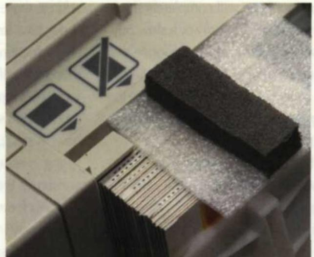
Adaptive piece of foam used to help scan cardboard mount in Nikon scanners
